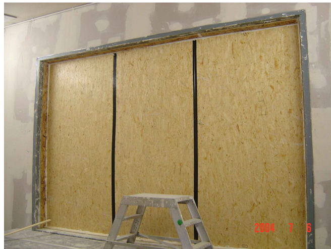
Photo 6 Kingspan Tek Panel System within test frame
