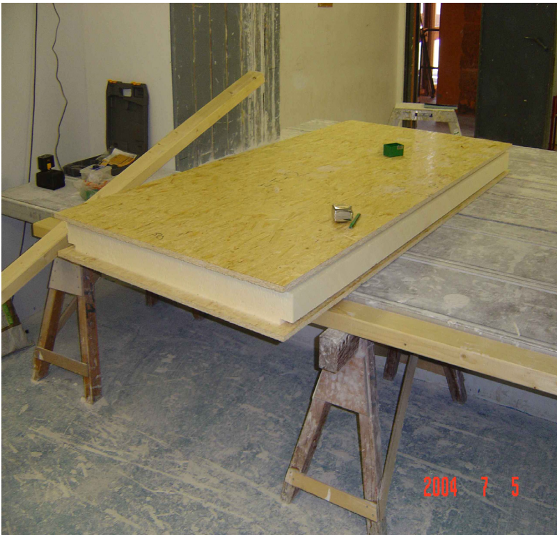
Photo 1 Single 142mm Kingspan Tek Panel
